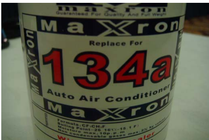
Picture 3: Refrigerant can labelled “Replace for 134a” but actually containing CFC-12
