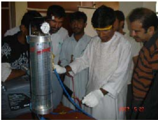
Participants performing the recovery of refrigerants and charging a system using dial-a-charge cylinder under the supervision of Mr. Kalantari, GTZ resource person (extreme right).
