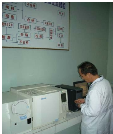
Photo: Chemist analysing water samples using Gas Chromatograph/Mass Spectrometer at the Jiamusi Environmental Monitoring Centre
